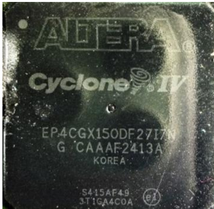
Figure 1. Field-Programmable Gate Array (FPGA)
