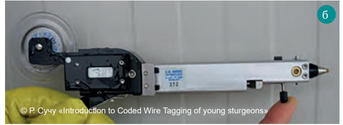
Image 27. T-Wand CWT detector (a), Multishot CWT injector (б)
