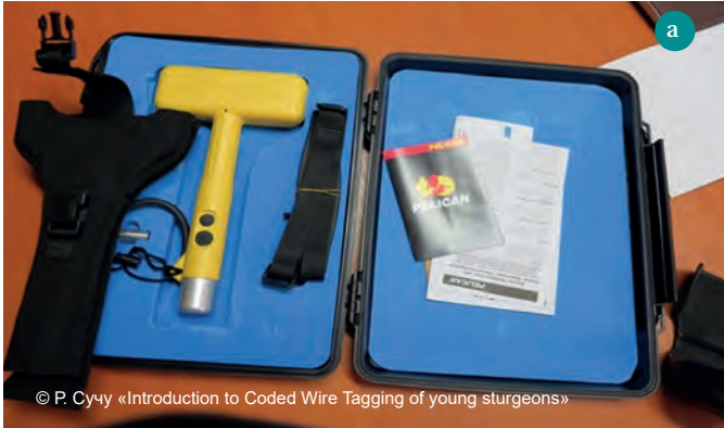
Image 27. T-Wand CWT detector (a), Multishot CWT injector (б)
