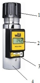
Figure 8. Wile-55 moisture meter: 1 – case cover; 2 – digital indicator; 3 – control panel; 4 – test sample container
