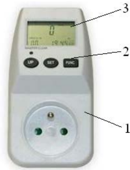
Figure 6. EMF-1 electronic wattmeter: 1 – wattmeter housing; 2 – control panel; 3 – indicator display
