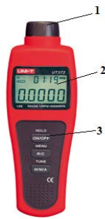
Figure 4. UNI-T UT372 frequency meter: 1 – laser reader; 2 – digital indicator; 3 – control panel
