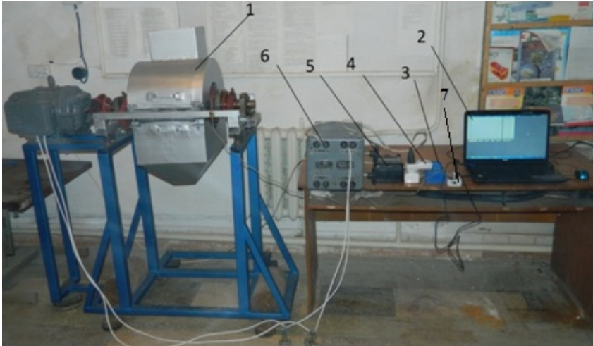
Figure 2. Experimental stand: 1 – experimental sample of the vibratory disk crusher; 2 – personal computer; 3 – switch; 4 – EMF-1 electronic wattmeter; 5 – secondary electromechanical wattmeter; 6 – AOCB-20-220-75 laboratory transformer; 7 – accelerometer
