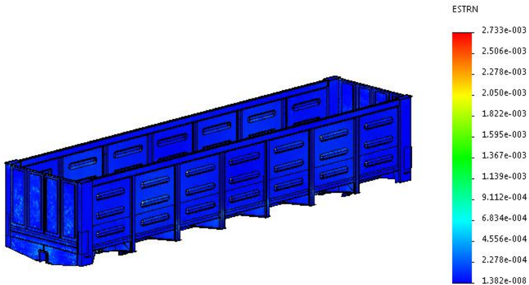
Figure 3.4. The results of the calculation of the load-bearing structure durability of the 12-757 model gondola wagon in rating condition I (impact)
