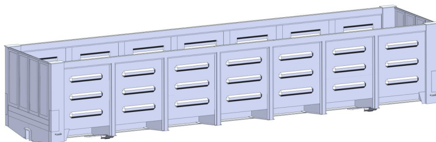
Figure 2.2. A spacial model of the load-bearing structure of gondola wagon
