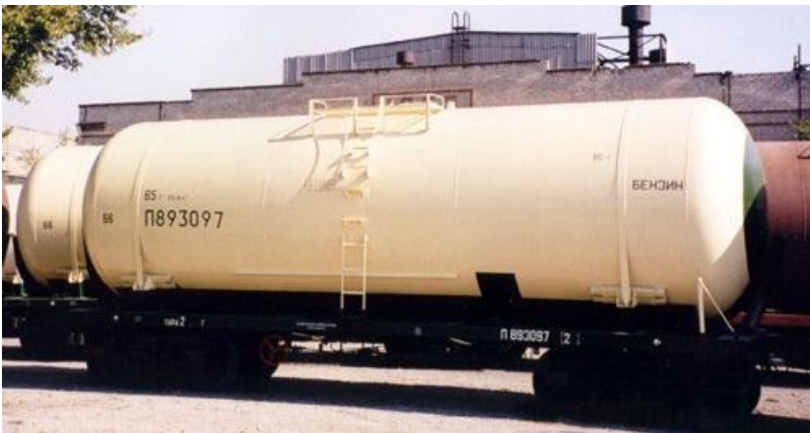
Figure 1.40. A 15-1443-06 model tank wagon for transporting light oil products
