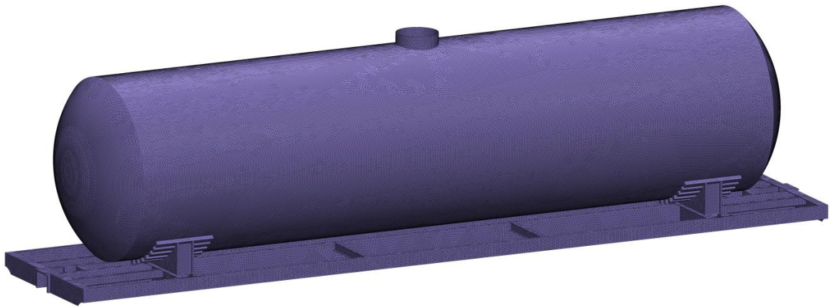
Figure 3.26. Finite element model of a tank wagon
