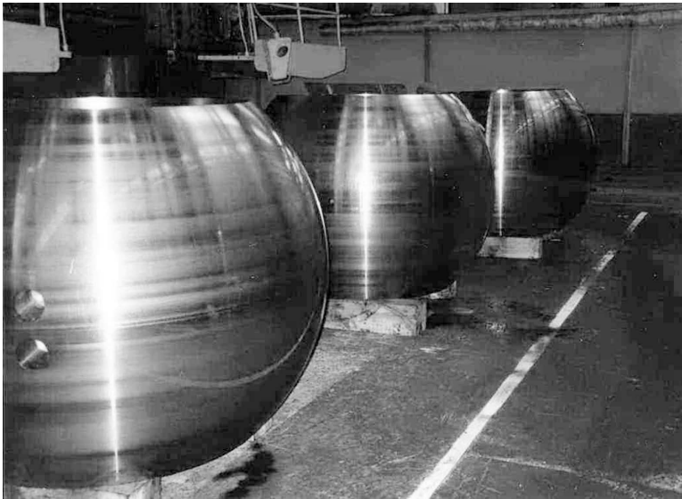
Figure 10.3 – Example of the forged piece after the sphere roughing
