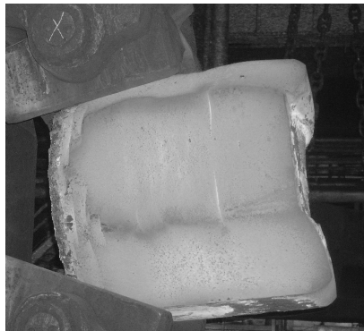
Figure 5.4 – Drawing the workpiece after groove formation in the end
