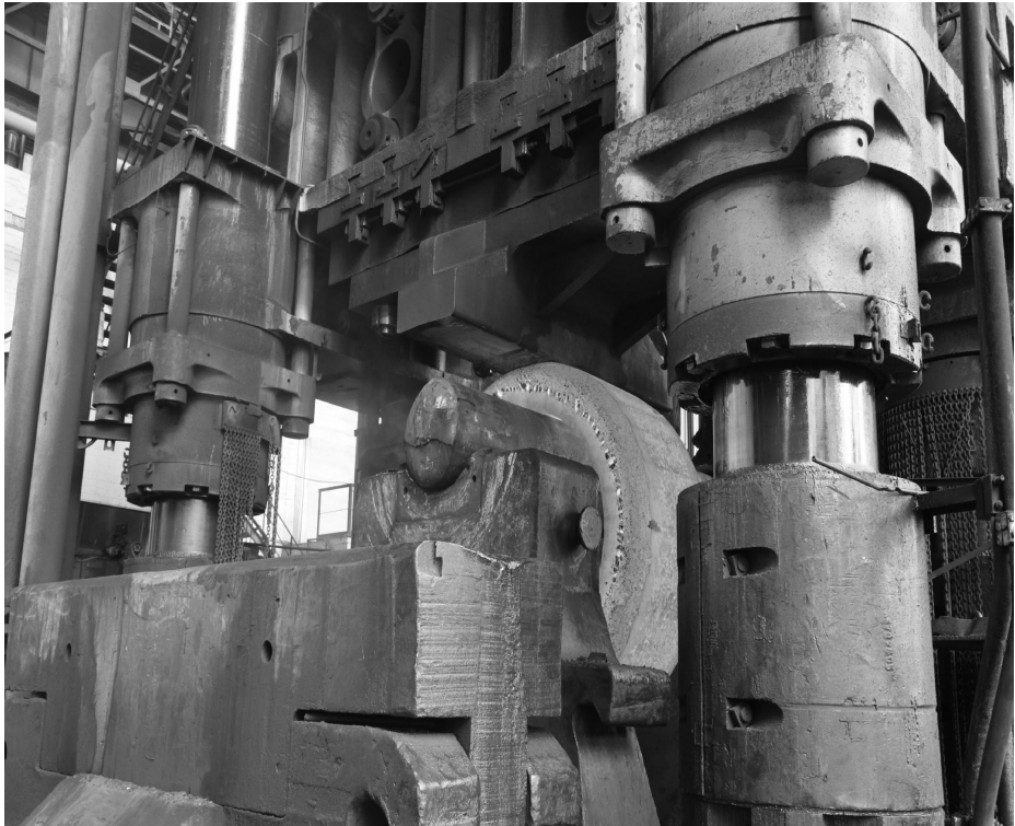
Figure 8.1 – Rolling-of the ring after the upsetting
