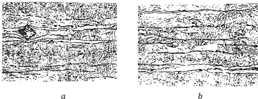
**Figure 3.17** – The microstructure of the steel 05X18H10T, the deformation martensite (microhardness  $H_{\mu}$  714)
