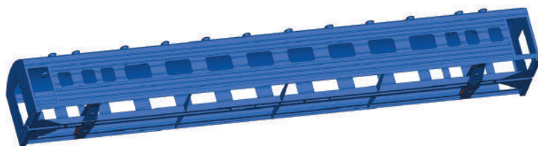
Figure 3.83 – Carrying structure of a passenger car with units for fixation on the deck
