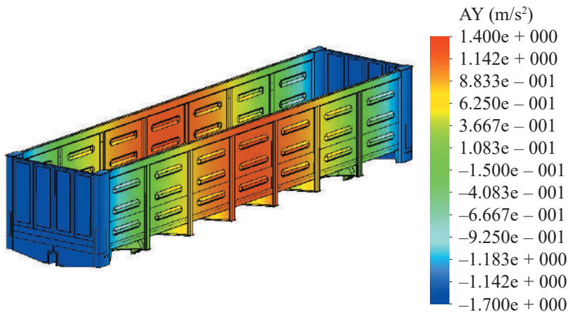
Figure 3.103 – Distribution of acceleration fields on the carrying structure of an open car body during viscous interaction with the ferry deck (bottom view)
