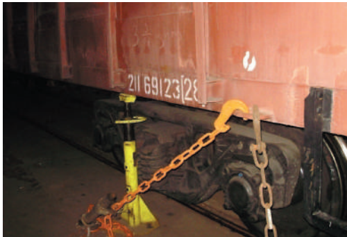
Figure 2.60 – Fixation pattern for a boxcar on the ferry deck
