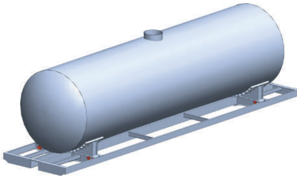
Figure 3.23 – Spatial model of the carrying structure of a tank car with units for fixation on the deck
