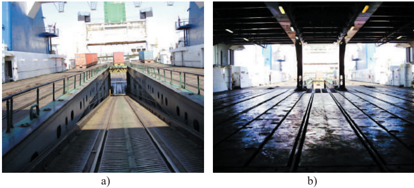
Figure 1.40 – Train ferry Greifswald : a) roll-on ramp; b) upper deck
