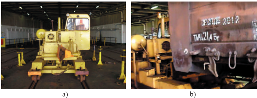
Figure 1.31 – Railcar mover (uniloc): a) in free state; b) in interaction with a car
