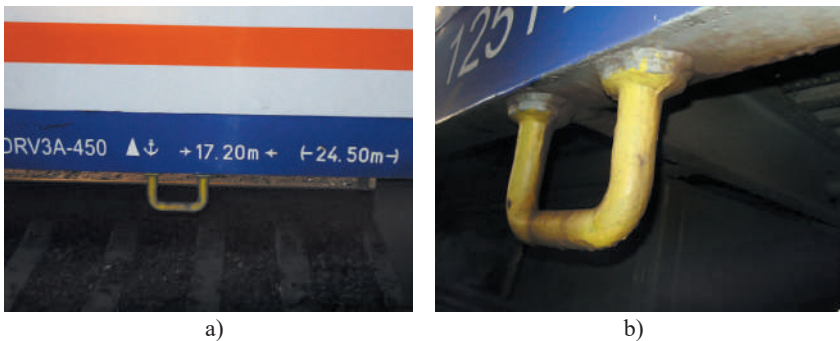
Figure 2.108 – Brackets for fixation of a passenger car body on the train ferry deck: a) front view; b) side view
