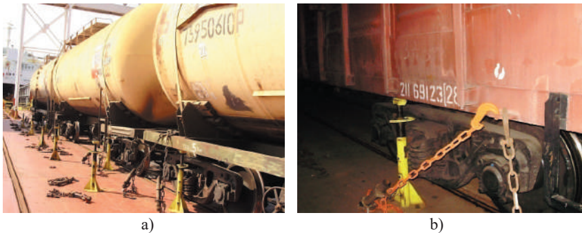
a) b) Figure 1.34 – Chain binders in operation: a) fixation of tank car; b) fixation of boxcar
