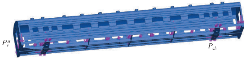
Figure 3.84 – Design diagram of the carrying structure of a passenger car at angular displacements relative to the transverse axle
