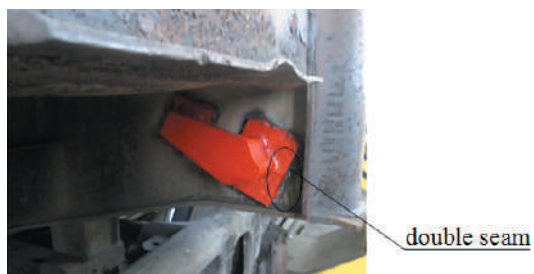
Figure 5.11 – Location of a unit for fixation of a chain binder’s hook on the bolster beam of an open car
