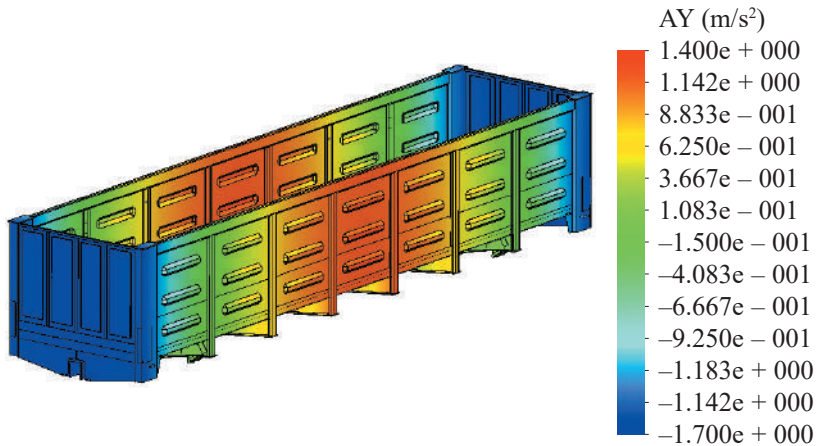
Figure 3.102 – Distribution of acceleration fields on the carrying structure of an open car body during viscous interaction with the ferry deck (side view)
