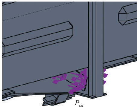
Figure 3.101 – Modelling forces through the device for fixation of a body on the deck
