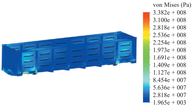
Figure 2.27 – Stress state of an open car body at angular displacements relative to the transverse axle
