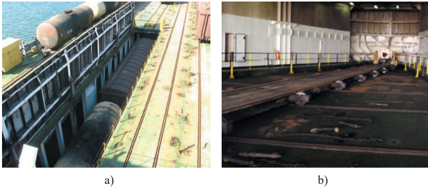
Figure 1.32 – Devices for transferring cars on the ferry deck: a) hydraulic elevator; b) rotating sector
