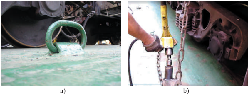
a) b) Figure 1.34 – Chain binders in operation: a) fixation of tank car; b) fixation of boxcar
