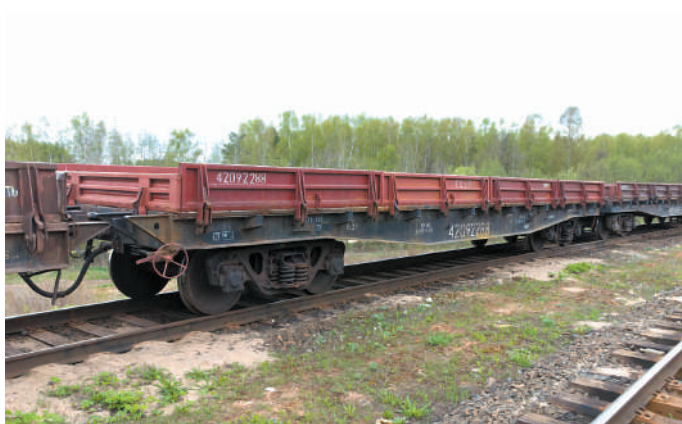
Figure 2.95 – Universal flat car of model 13-401
