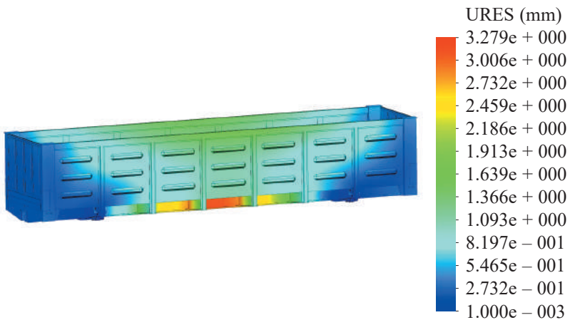
Figure 3.12 – Displacements in the units of an open car body at angular displacements relative to the transverse axle
