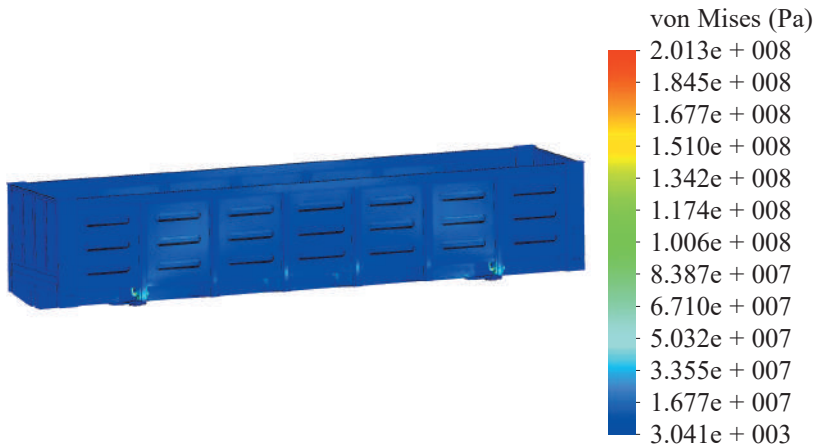
Figure 3.9 – Stress state of an open car body at angular displacements relative to the transverse axle
