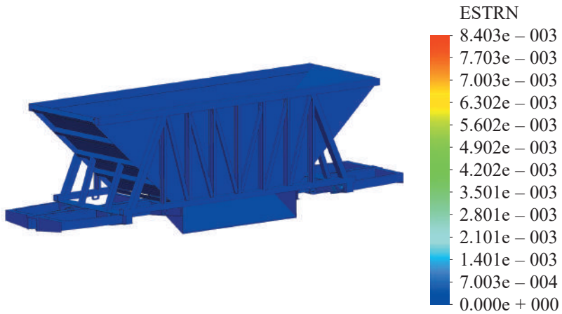
Figure 3.62 – Deformations in the carrying structure of a hopper car at angular displacements relative to the transverse axle
