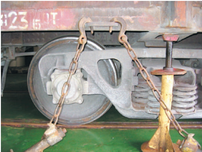
Figure 2.22 – Fixation of an open car on the ferry deck
