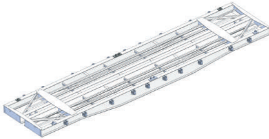
Figure 2.96 – Carrying structure of a 13-401 flat car
