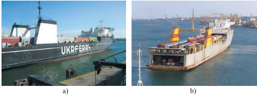
Figure 1.18 – Rail cars on upper decks of ferries: a) Geroi Shipki ; b) Geroi Odessa
