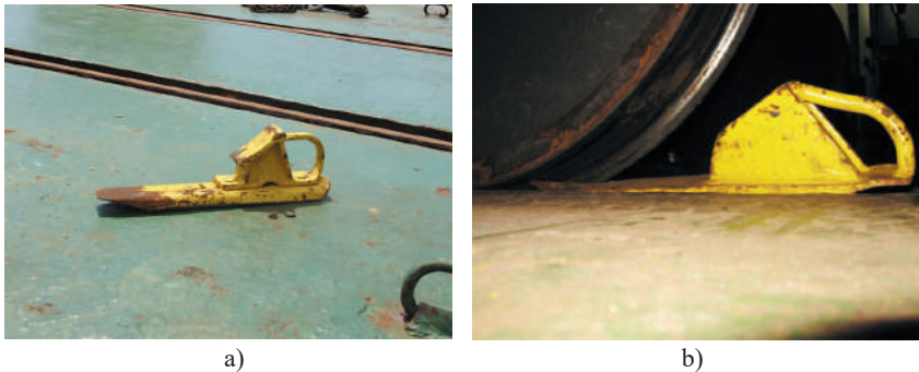
Figure 1.38 – Brake shoes: a) in free state; b) under the car wheel
