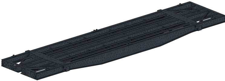
Figure 3.74 – Finite element model of the carrying structure of a flat car with units for fixation on the deck
