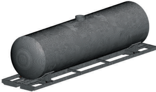
Figure 3.26 – Spatial model of the carrying structure of a tank car with units for fixation on the deck
