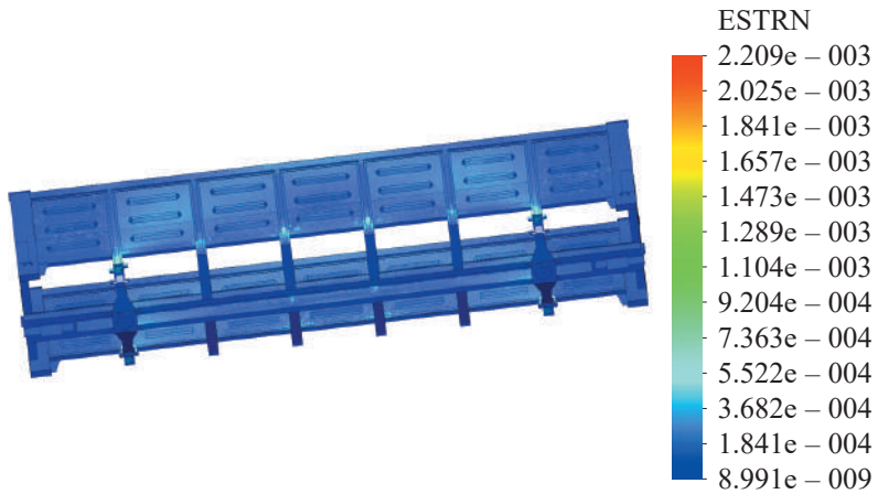
Figure 3.15 – Deformations in the open car body at angular displacements relative to the transverse axle
