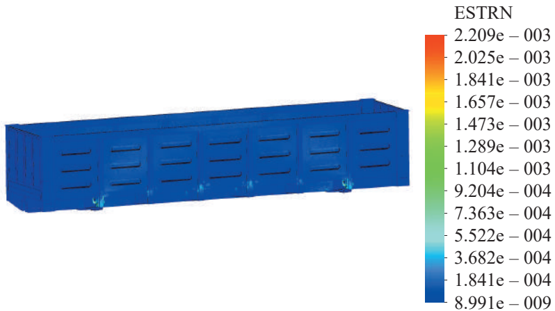
Figure 3.14 – Deformations in the open car body at angular displacements relative to the transverse axle
