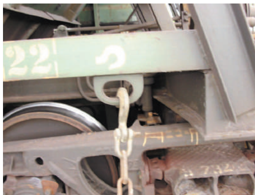
Figure 2.77 – Fixation pattern for a hopper car on the ferry deck
