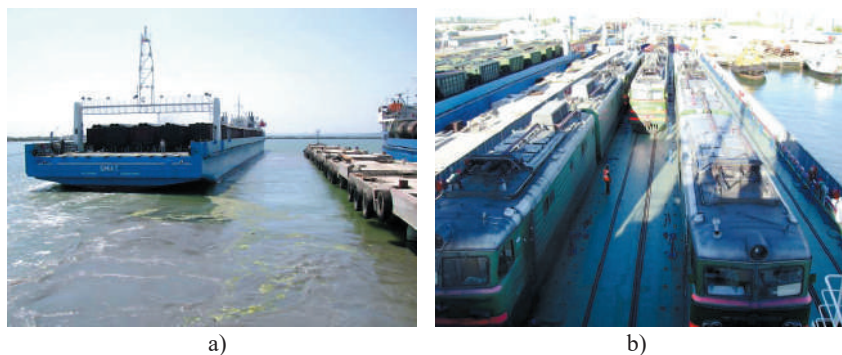
Figure 1.17 – Train ferry SMAT : a) loaded with open cars; b) loaded with traction rolling stock
