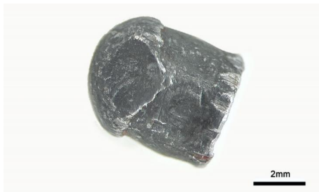
Fig. 6. A bullet with slight deformation on the surface of the semi-spherical head portion. Macrophoto
