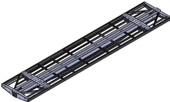
Figure 3.55 – Spatial model of the bearing structure of the flat wagon
