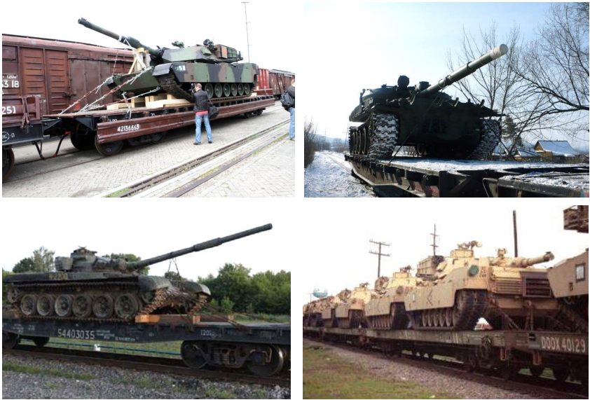
Figure 3.45 - Tanks secured on flat wagons
