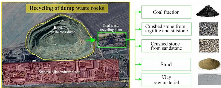
Figure 1. Generalized conceptual scheme for producing the main resources during the recycling of waste rock from the Stepova mine dump
