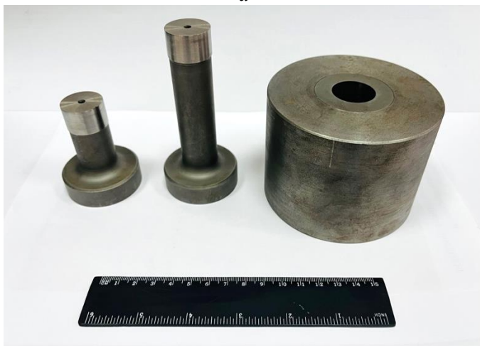
Fig. 2.2. Molds for pressing cylindrical samples
