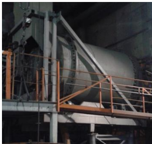
Fig. 1. Rotary gas melting furnace
