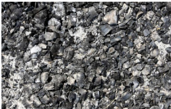
Figure 2. Inadequately burned cinder
