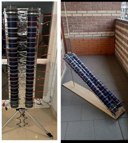
Fig. 1. Experimental CCPVM setup with liquid cooling for simultaneous electrical and thermal energy generation
