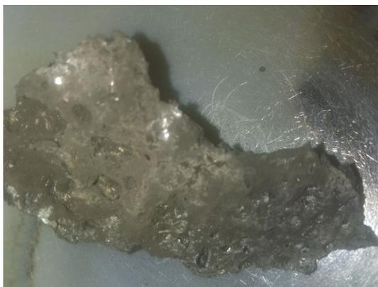
**Figure 4. Dry residue after nitrate pyrolysis**
