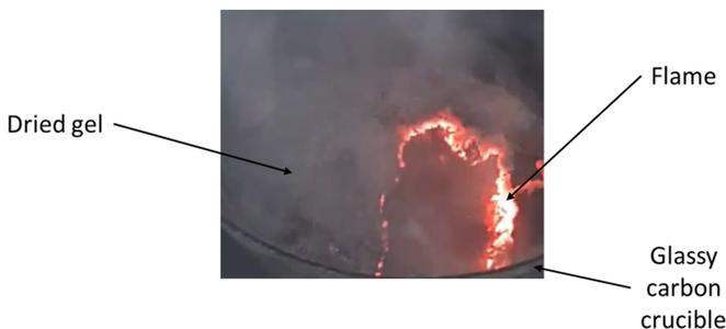
**Figure 3. Combustion reaction of a nitrate-citrate precursor**
