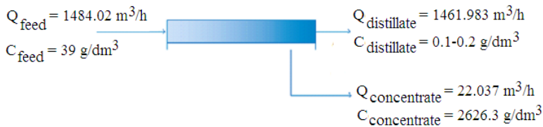
Fig. 6. Balance sheet of the mine water desalination process using the proposed ZLD technology
