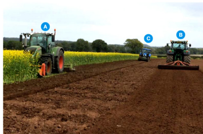
Figure 2.8.2 – Multiple-pass biofumigation system: tractor A flail topping and shallow rotavating, followed by tractor B ploughing to 30 cm, followed by tractor C power-harrowing with packer-roll.
