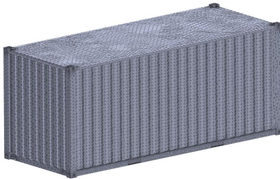
Figure 3.59 – The finite element model of the container
