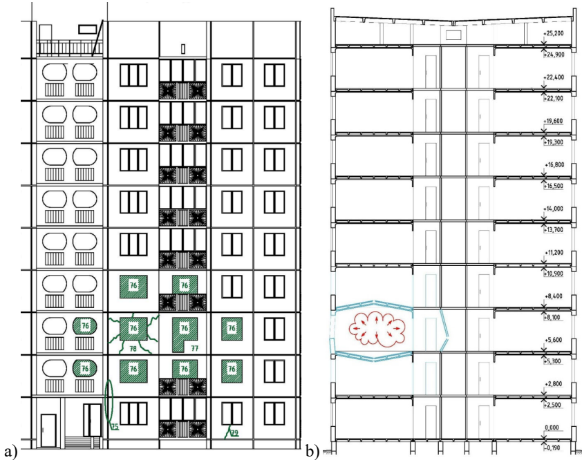
Figure 4.5 – Location of damage to reinforced concrete structures: a) fragment of the facade; b) cross-section of the building
