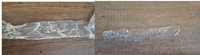
Fig. 7. Swelling of experimental films № 4 and № 5
